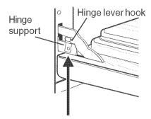
Lock engaged for door removal Figure 1
